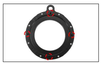
Locate the 4 small sockets of the M67 mounting ring. Align with the positioning pins on the MWL-1 and place it on top.
